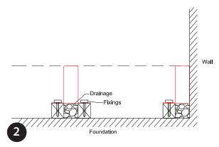
Fix housings to spaces with suitable fixings.
