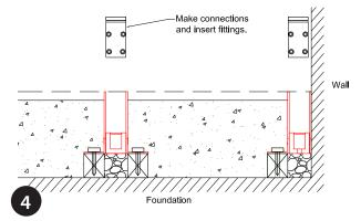
Make product power connections ensuring they are appropriate for the environment, pack cables into housing ensuring that no stress or pinching occurs as product is fitted into housing. Ensure product is pushed fully into housing clips.
